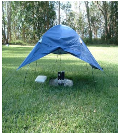
Fig. 2. A close up of a playback unit, showing the speakers, tent and coreflute. The digital audio player and connection to the power was housed in the white plastic container.
